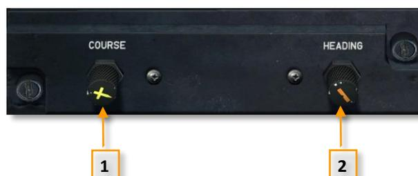
Figura 3-78 Panel de control remoto del HSI
